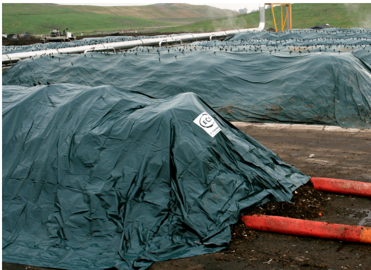
The CompDogs are buried underneath the piles and later removed forming the aeration vault. The CompDog™ is deployed and retrieved using Dog Rollers.
