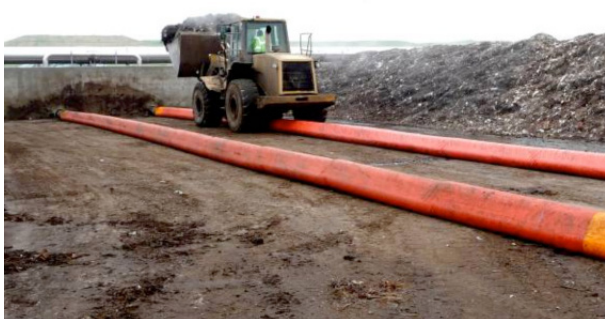
The CompDogs are buried underneath the piles and later removed forming the aeration vault. The CompDog™ is deployed and retrieved using Dog Rollers.
